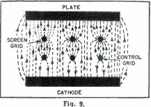
trons than there should be in normal diode operation. If the grid is positive enough, the electrons can be imagined to be replaced by positive ions. This enables the plate to affect electrons much deeper in the space charge, and since the grid serves only to neutralize or to partially neutralize the shielding effect of the electrons under their influence while these electrons are continuing their motion towards the plate, the plate current will consequently be increased.
