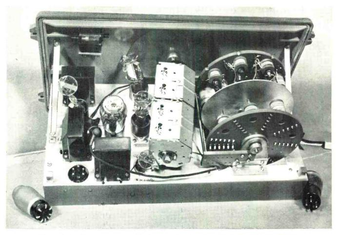
This smashed up all-wave receiver was taken from a torpedoed ship and arrived at the shop in this condition.
