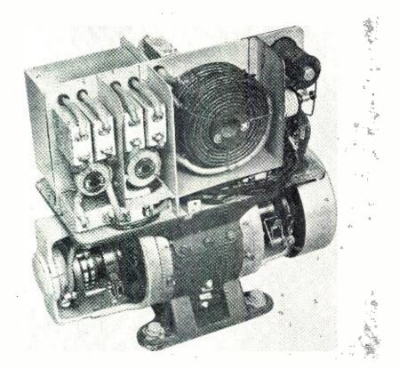
Power Unit and associated filter circuit components for the transmitter and receiver removed from Nazi aircraft.
