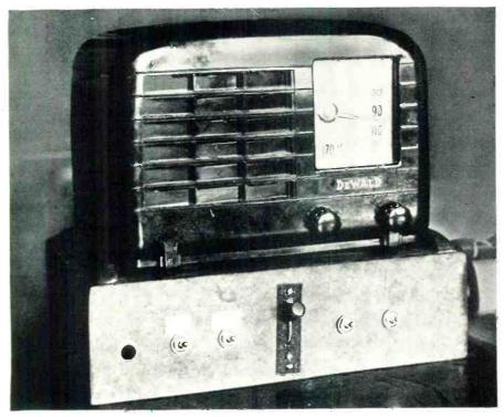
Front view of the Master Station, built from DeWald midget receiver.
