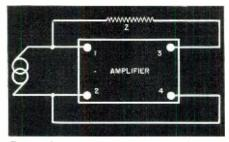
Fig. 2. How negative resistance is obtained.
