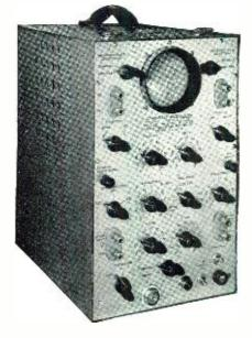
panel of the unit. The Y-amplifier has an input connection for the Shielded-Cable Test Probe Type 242A, supplied with the instrument. This reduces input capacitance and eliminates stray pickup. All high-voltage electrolytic condensers are eliminated from circuit.
