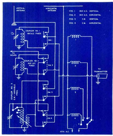
An elaborate antenna coupler was designed for the special transmitters.
