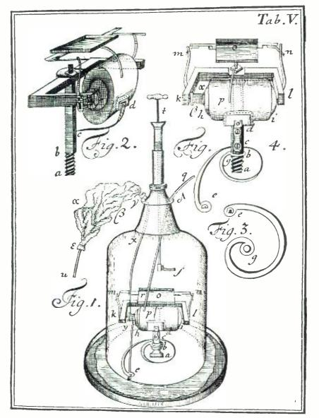
Fig. 3. Details of Winkler's Machine. Fig. 1 shows the ma. chine set up for operation within a vacuum in glass jar.
