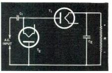
Fig. 1. Half wave voltage-doubler.
