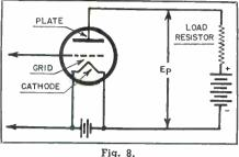
pable of influencing the motion of electrons within the tube while at the same time the grid, due to the small area of metal present, will allow electrons to move more or less freely without striking the metal part of the grid if the plate is operated at a much higher positive potential than the grid.
