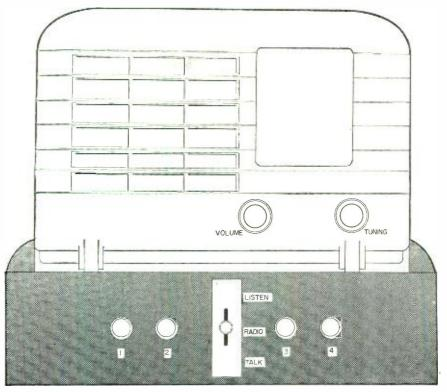
Front view and layout for the Master Station. A three-position vertical switch is centered on the front of the sub-chassis.
