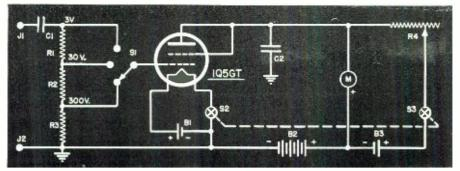
Fig. 3. An easily-built battery-operated VTVM uses only 1 tube.
