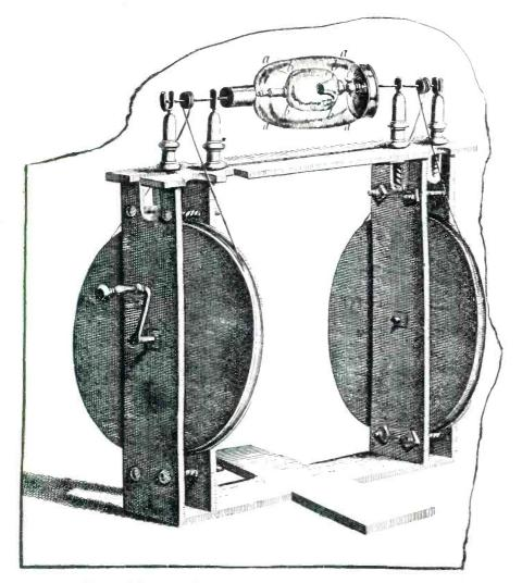
Fig. 2. Cylinder Machine as used by Hauksbee in his early experiments. Note the belt drive to increase speed of rotating elements.
